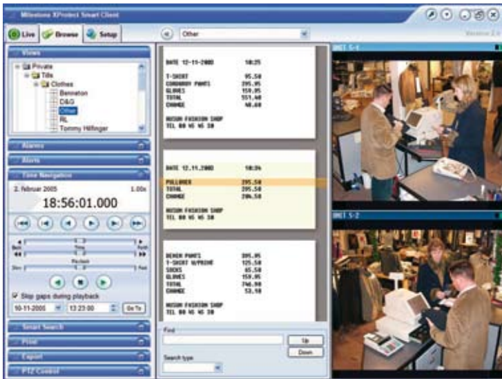
Figure 11.4a An example of a PoS system integrated with video surveillance. This screenshot displays the receipts together with video clips of the event. Picture courtesy of Milestone Systems.
